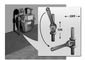
It is a quarter turn valve and in order to turn the flow off, the tab needs to be turned so that it is cross wise to the flow.
